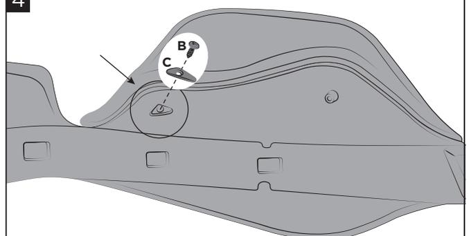
**Drill a preliminary hole to ease the centering of the screw.**
