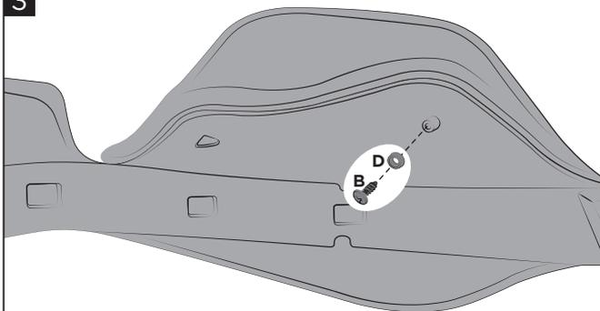
**Tighten the spoiler using screw (B) and bushing (D).**
