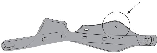
**Drill a hole of 8mm on the cover, as shown in figure.**
